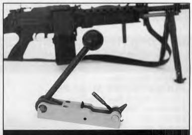
Those who intend to reload using surplus military cases, which almost always have primers that are staked or ring-crimped in place are well-advised to obtain the Dillon Super Swage 600, a tool designed specifically to remove the crimp and permit a new primer to be properly seated in the pocket.
